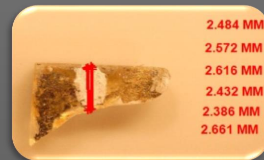
Figure 3: Prepared sample of TGS White Crystal Scale: Millimeters
