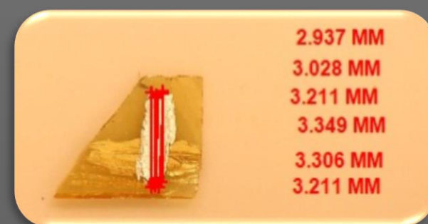
Figure 1: Prepared sample of BTO Yellow Crystal Scale: Millimeters
