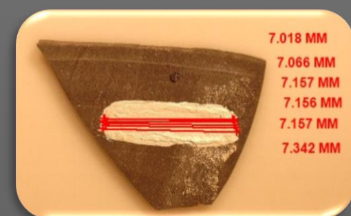
Figure 2: Prepared sample of BTO Grey Ceramic Scale: Millimeters
