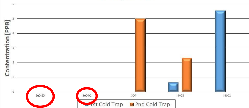
Concentration of Molecular Compounds on College of the Desert Air Cold Traps in Series
